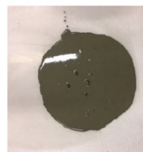
Cement paste with superplasticizers (Polycarboxylate)
