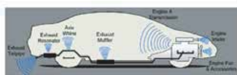
Powertrain Airborne Noise Sources
